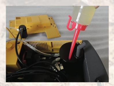
Once the tank is open, you may begin to fill up the oil. We recommend using a toothpick or something similar to gauge the oil level. For the first oil fill, add less than 150ml of oil and let the excavator run for a while. Then proceed to add an additional 80ml of oil. Close the tank immediately after.
