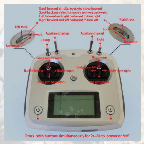
Important Note: All switches must be kept in the up position while turning on the radio. Otherwise, there will be a continuous warning sound.
